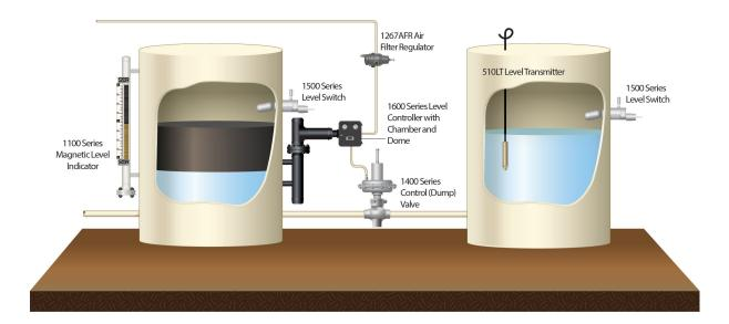
SENSOR can provide SOR Submersible Transmitters to measure level in an open tank, or SOR model 815DT Differential Pressure Transmitters for pressurized or floating roof tanks.
