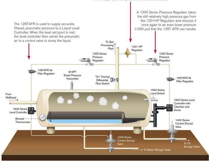
The 1201 High Pressure Regulator is designed to provide pressure control in numerous processes that involve a high-pressure drop. It is an extremely durable regulator capable of handling a max inlet pressure of 5000 psi (345 bar). The spring configuration of the 1201 Regulator can be configured to provide five different outlet pressures ranging from 0-225 psi (0-15.5 bar).
